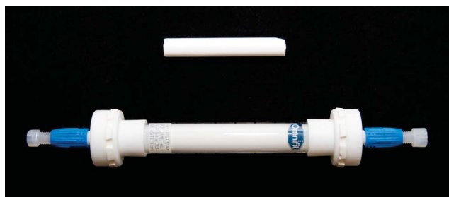
Fig. 1 Monolithic triphenylphosphine reagent, with and without glass column housing.
